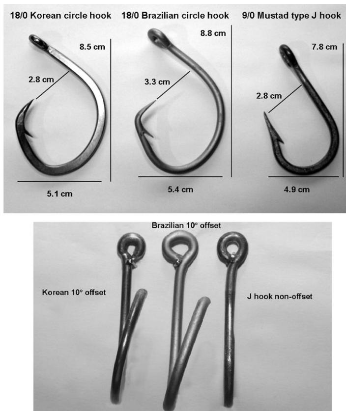
Figure 2. Lateral (above) and frontal (below) views of circle hooks 18/0, 10° offset (Korean – left, Brazilian – centre) and Mustad type ‘J’ hook 9/0, 0° offset – right. Photos: V. Fonseca.
